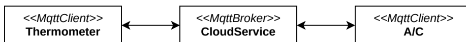
Figure 5.3.: The central MQTT broker relays messages to subscribed clients. In this case, the A/C unit receives messages published to a topic it subscribed to.
